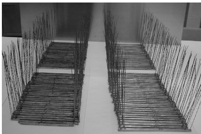
Fig. 1. Samples used for the resistance measurements with the spark welded copper probes for the four-point method measurements.
